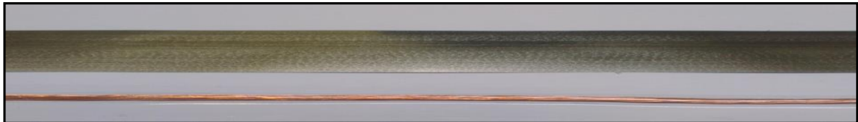
Amorphous heating material in comparison to traditional heating wire.
