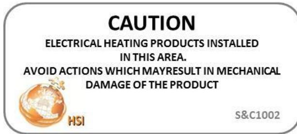
S&C1002 To be affixed to the location of the installed electrical roof heating cables
